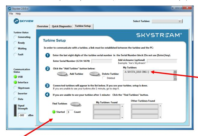
Within the 60 seconds, the turbine serial number should show up in the "My Turbines Found" field
