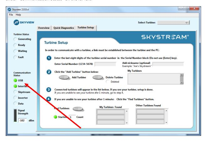
Now you can proceed with entering your serial number in the Turbine Setup screen under step 1. Once the 8 digit number is entered there, click "add turbine" under step 2
