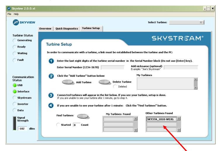
To get it to "jump" over to "My Turbines Found" simply go to the File menu in the upper left corner of the screen, and click on "Disconnect from USB Converter"
