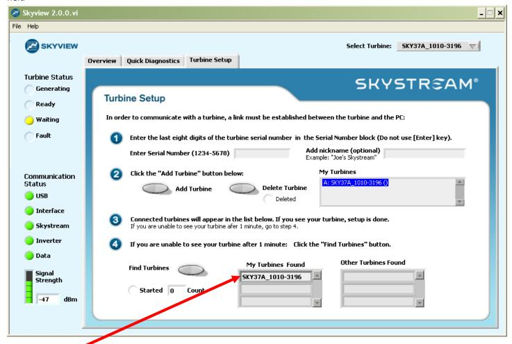
Occasionally the interface will "find" the turbine before you have a chance to enter the serial number, in which case the serial number will show up in an encoded format under "Other Turbines Found"
