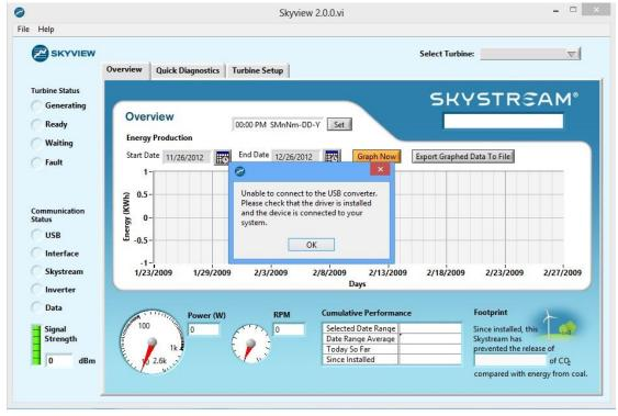
If your Skyview screen looks like this or the image below, with no green lights under "Communication Status" in the far left of the screen, this is another indication that the drivers for the xBee interface have not loaded.
