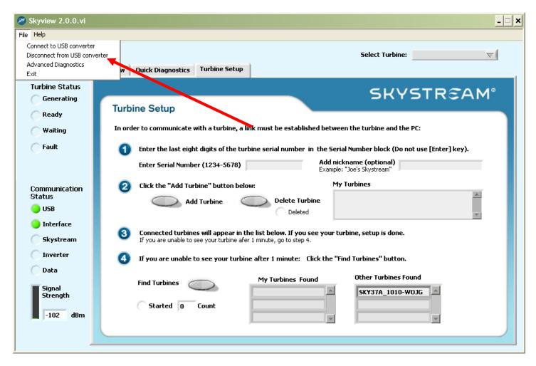
The USB and Interface lights will go out. As soon as they do, click on File/Connect to USB Converter. The turbine's serial number will "jump" over to the My Turbines Found field and you will notice all five Communication Status lights will be green:
